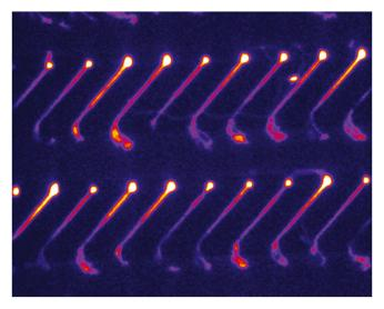
**Movie S1.** Parking and loading of T4 DNA molecules to form a plethora of DNA dumbbells is shown. DNA molecules are parked in molecular gates, which are abutted next to nanoslits, under a low voltage ( $V_p = 20$  V). DNA molecules are triggered to load at a higher voltage ( $V_L = 70$  V) to form dumbbells. Original movie duration is 70.0 s (~214 ms per frame), but is compressed here to run 4.38× faster; movie field is 26.9 × 21.3 µm.
