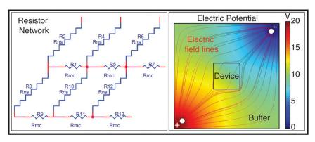
**Fig. S1.** (*Left*) Resistor network approximation for nanoslit–microchannel network. Unit cell consists of one resistor representing microchannel resistance and one resistor representing the nanoslit. The value of the resistors can be obtained from 1D narrow electrolyte channel model involving Poisson–Boltzmann and Navier–Stokes system of equations. (*Right*) Potential and electric field lines within the device and tank when a potential difference of 20 V is applied.
