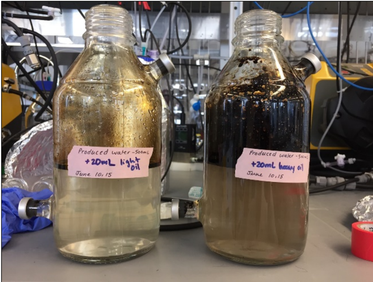
Figure S-2. Image of the light (left) and heavy (right) oil cultures prepared in modified 1-L serum bottles.
