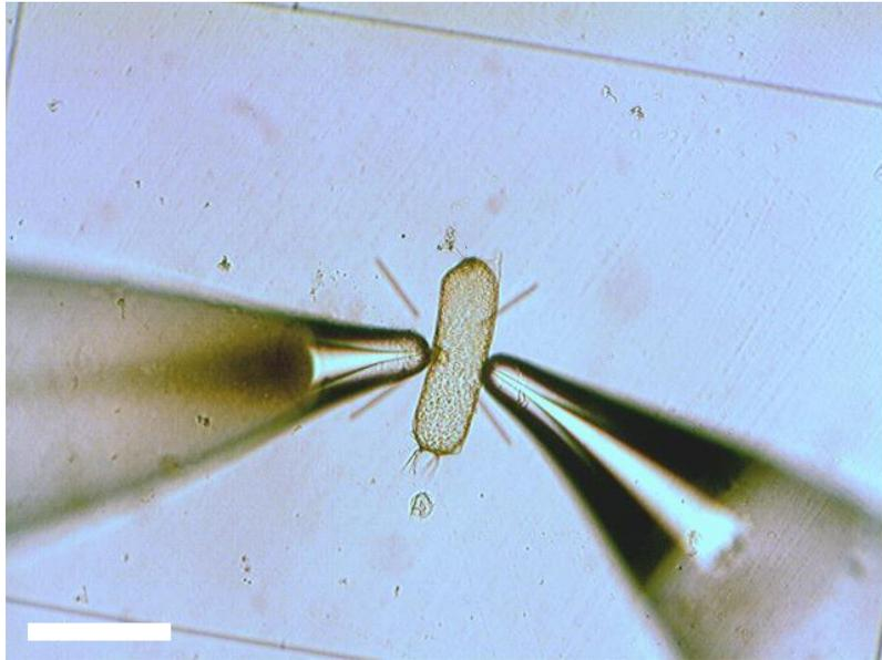
**Supplementary Figure 5: Positioning of microelectrodes around an *O. sinensis* cell for simultaneous measurement of pH and  $\text{CO}_3^{2-}$**
