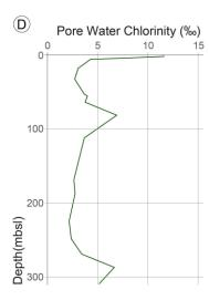
Distribution of the chlorinity of pore water at the DSDP hole 379A in the central plain of the Black Sea (modified from Merey and Sinayuc, 2016 and Calvert and Batchelor, 1978). This figure was integrated to the Supplementary Fig 2.
