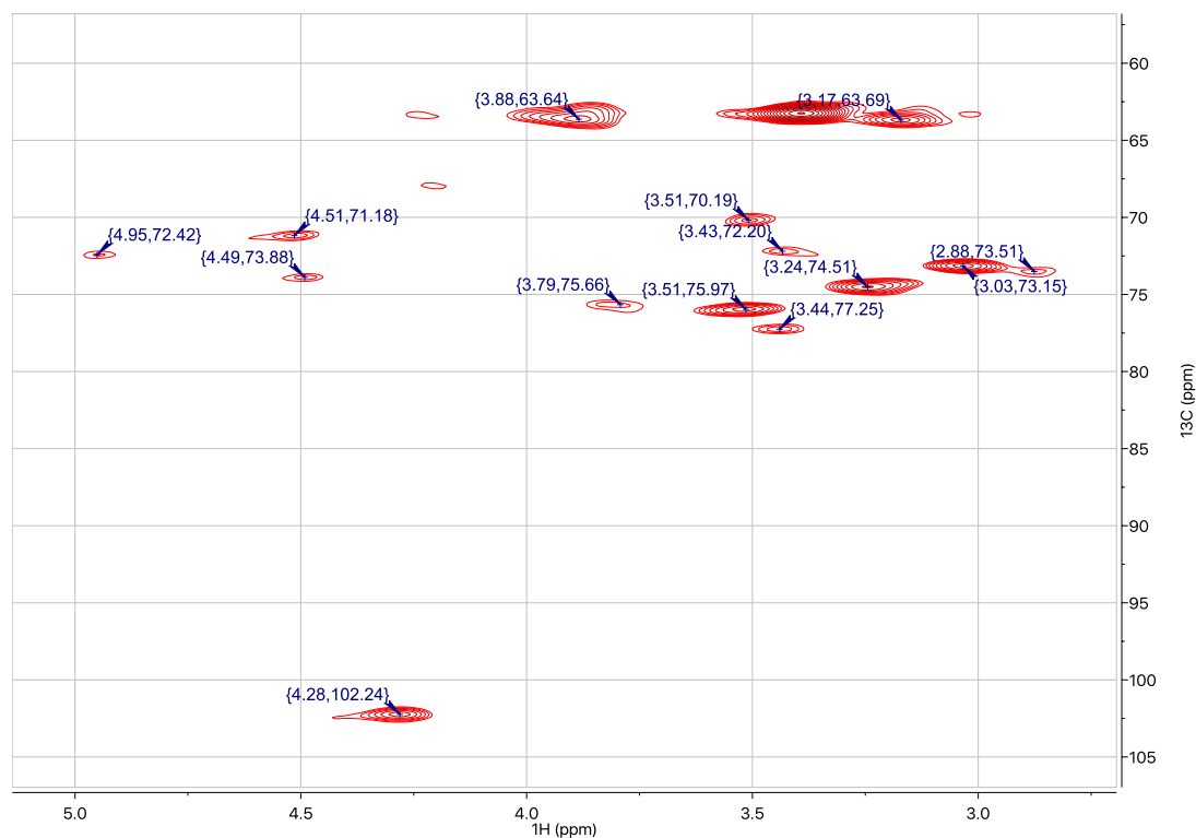
SF7. Multiplicity-edited HSQC spectra for AcNFC extracted with DMSO- d_6 , recorded at 40 °C.
