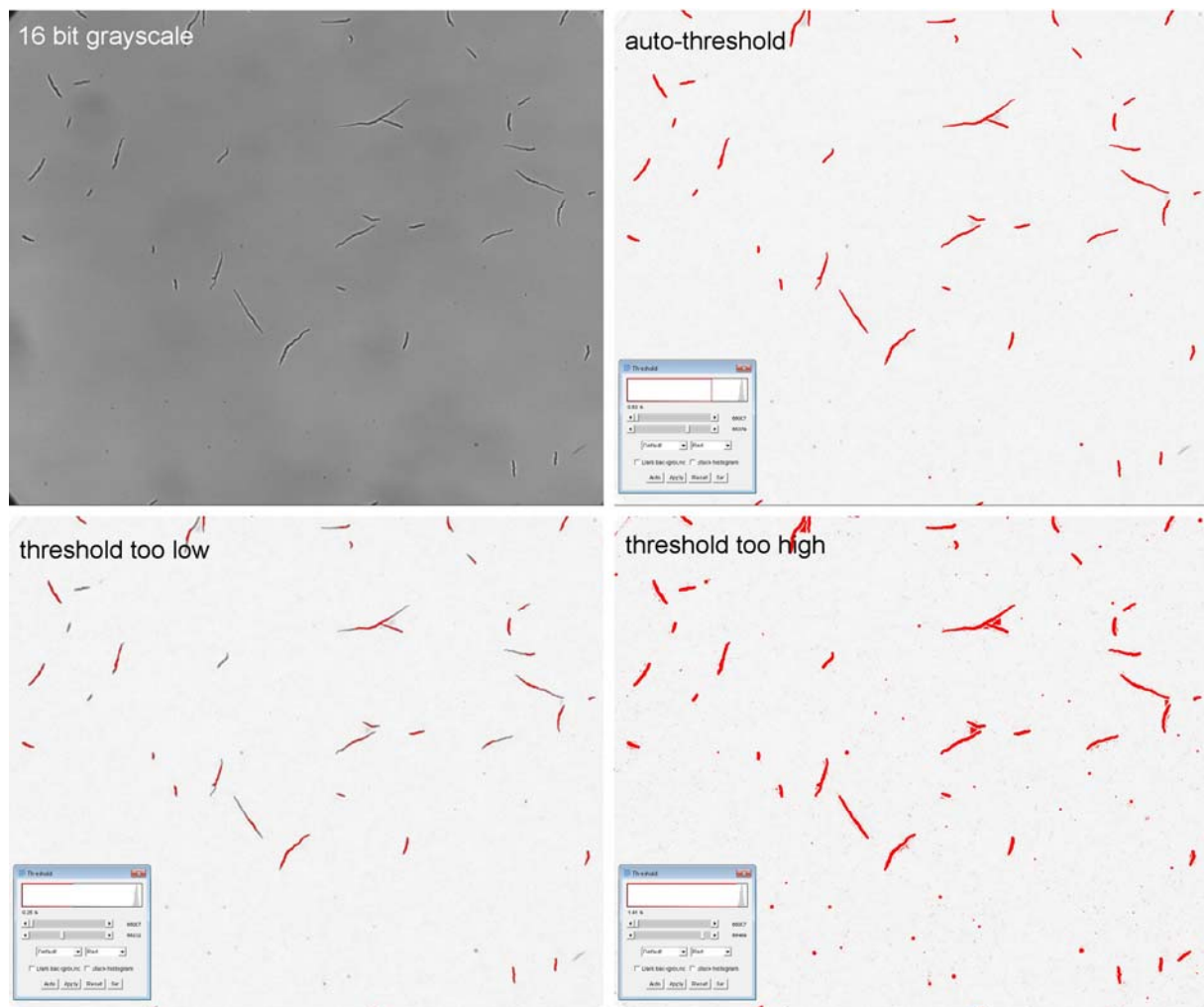
Fig. S9. Importance of the threshold during the Create binary image routine. In most cases using the 16-bit grayscale image stack (left, top) the default auto-threshold will end up with a satisfying result by rejecting most of the non-spore particles while fully representing the actual spores (top, right). If the threshold is set too low (bottom, left), the areal space of spores might not properly be filled and less spores and background particles might end up in the analysis. In contrast, when the threshold is set too high (bottom, right), it will result in further shading of non-hyphal areas like shadows, scratches and air bubbles.
