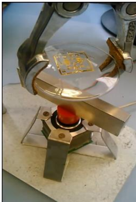
fig. S4. Angle characterization setup. A permanent bar magnet is attached to the shaft of a stepper motor to provide a constant field in the plane of the 2D sensor. The sensor is fixed on a curved glass support suspended over the magnet such that the in-plane field magnitude is 50 Oe. Upon rotation of the magnet the angular response of the sensor is monitored at a computer.
