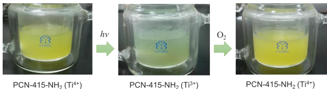
Figure S26. The color change of the reaction suspension upon light irradiation in the presence of N_2 and quickly back upon exposure to O_2 .
