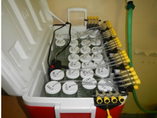
Figure S3. Experimental setup for a single temperature treatment, with 20 jars each containing an E. depressus , fit with an airstone connected to an aerator. To maintain a constant temperature for the whole cooler we placed a single pump head next to an aquarium heater.
