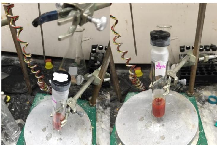
**(Left)** Removal of Ar balloon and covering septum with Teflon™ tape. **(Right)** Covering the Teflon™ tape with electrical tape.
