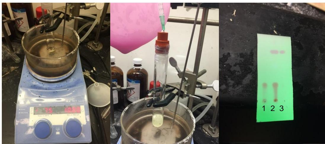
(Left) The vial was put in a preheated 75 °C oil bath. (Center) After heating for 30 min. (Right) TLC (hexanes/ethyl acetate 2:1) under UV indicates completion of the redox-active ester formation. Lane 1: starting material of TCNHPI; Lane 2: co-spot of starting material and reaction mixture; Lane 3: reaction mixture.
