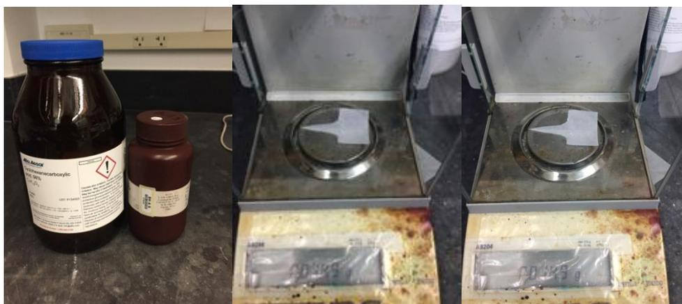
**Left:** Carboxylic acid and HATU. **Center:** Weight of carboxylic acid. **Right:** Weight of HATU.
