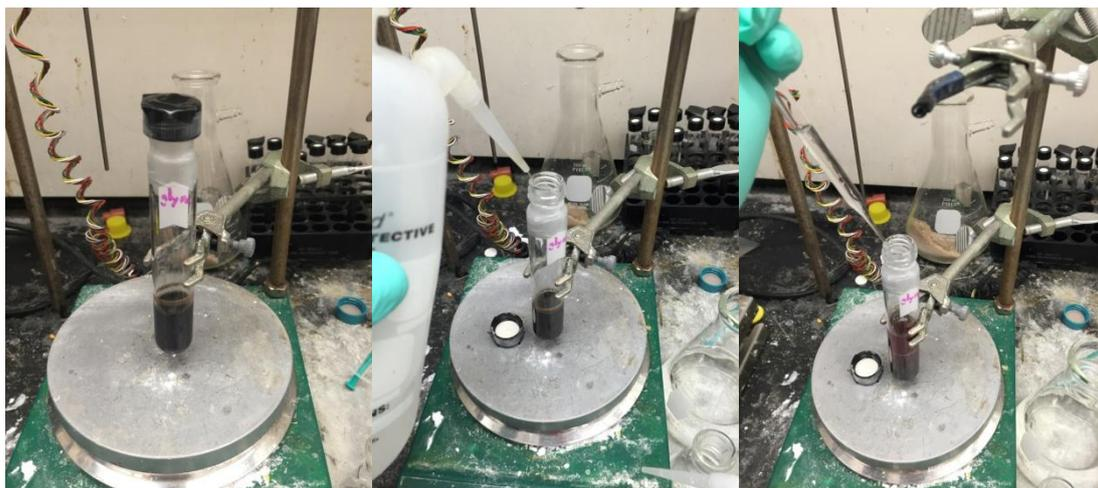
**(Left)** Reaction with  $\text{NiCl}_2\cdot\text{glyme}$  after 12 h. A black color is often observed but is not imperative to the success of the reaction. **(Center)** Dilution with  $\text{Et}_2\text{O}$ . **(Right)** Slow addition of 1M  $\text{HCl}$  (aq).
