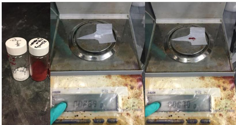
**Left:** Redox-active ester and catalyst. **Center:** Redox-active ester weight. **Right:** Fe(acac)<sub>3</sub> weight.
