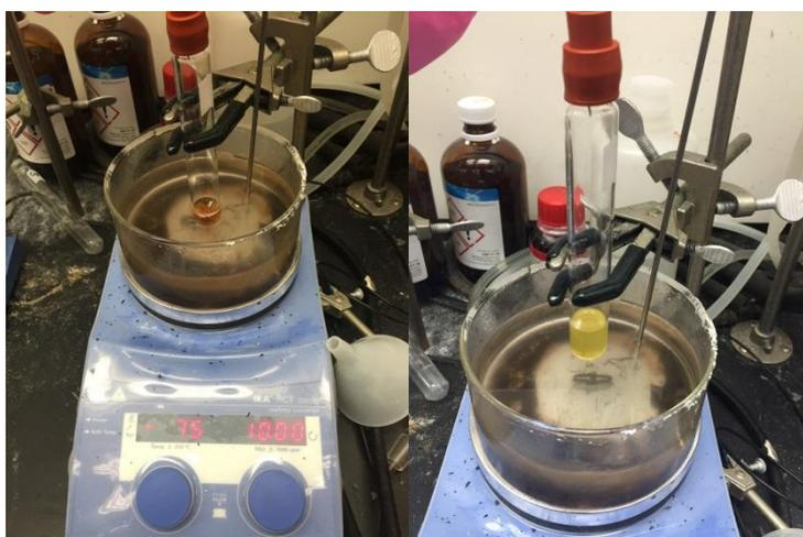
**(Left)** After heating for 5 min, the reaction mixture turned red. **(Right)** Reaction mixture after stirring for 12 h.
