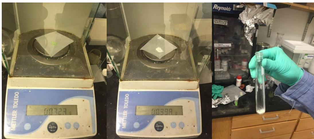
**(Left)**  $\text{NiCl}_2 \cdot 6\text{H}_2\text{O}$  (72 mg). **(Center)** bathophenanthroline (100 mg). **(Right)**  $\text{NiCl}_2 \cdot 6\text{H}_2\text{O}$  and bathophenanthroline in vial.
