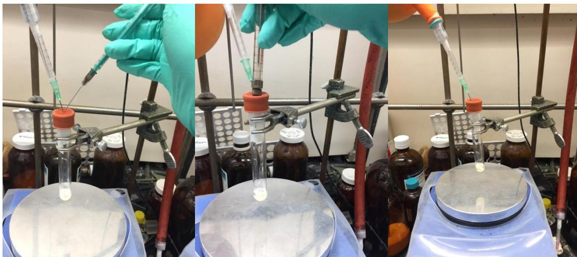
**(Left)** Addition of DMF. **(Center)** Addition of  $\text{Et}_3\text{N}$ . **(Right)** After addition of  $\text{Et}_3\text{N}$ , mixture becomes homogenous.
