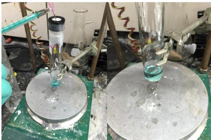
**(Left)** Blue color develops as the DMF solution is added. **(Right)** After all of the redox-active ester solution has been added and stirred for 5 min.
