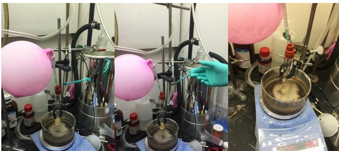
**(Left)** Add  $\text{Et}_3\text{N}$  (0.14 mL). **(Center)** Add  $\text{NiCl}_2 \cdot 6\text{H}_2\text{O}$ /bathophenanthroline stock solution (0.4 mL). **(Right)** Place the vial in a preheated  $75^\circ\text{C}$  oil bath immediately.
