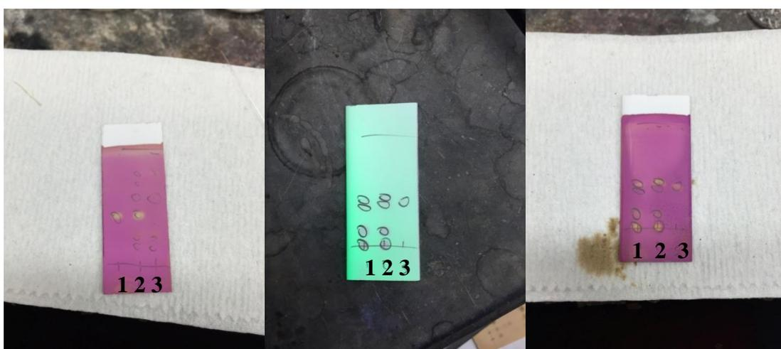
**(Left)** TLC (4:1 hexanes:ethyl acetate). Lane 1: redox-active ester; Lane 2: Co-spot; Lane 3: Reaction mixture **(Center and Right)** TLC (9:1 hexanes:DCM) Lane 1: Reaction mixture; Lane 2: Co-spot; Lane 3: Authentic sample of product.
