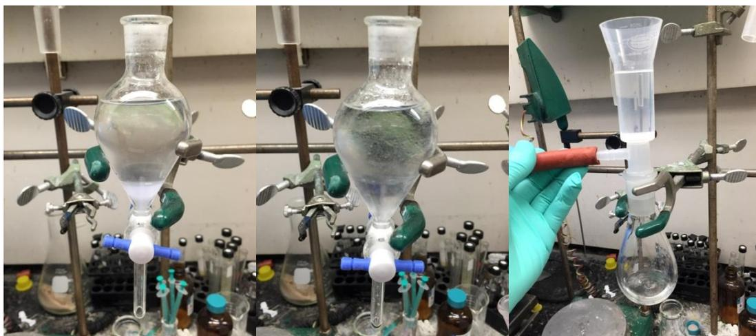
**(Left)** After 1M  $\text{HCl}$  (aq) wash. **(Center)** After  $\text{NaHCO}_3$  wash. **(Right)** Filtering the drying agent.
