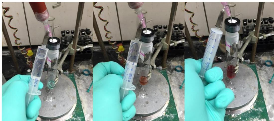
**(Left)** Prior to addition of ArylZnCl·LiCl. **(Center)** A red/brown color is immediately evident. **(Right)** Completed addition of ArylZnCl·LiCl solution.
