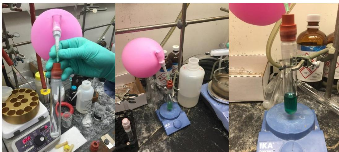
**(Left)** The flask with a stir bar was sealed with a septum, wrapped with parafilm, evacuated under vacuum and refilled with argon. This was done 3 times in total. **(Center)** Add DMF (6 mL) into the vial. **(Right)** After stirring for 3 h at r.t.
