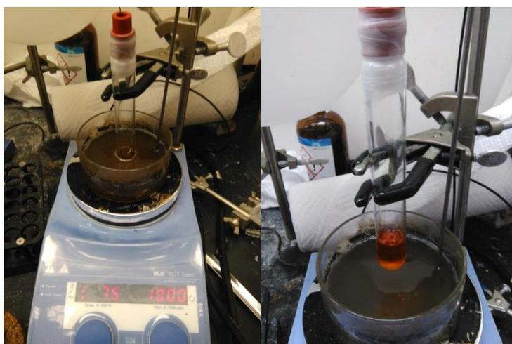
**(Left)** After addition of Ni/ligand complex, directly placed in preheated 75 °C oil bath. **(Right)** 5 min after heating, the reaction mixture turns red. **Note:** *the red color changing is crucial for the success of the reaction.*
