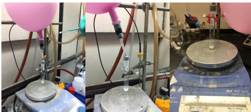
**Left:** Addition of THF. **Center:** After addition of THF (white suspension). **Right:** Solution after 2 h stirring at r.t. (it becomes a clear solution).
