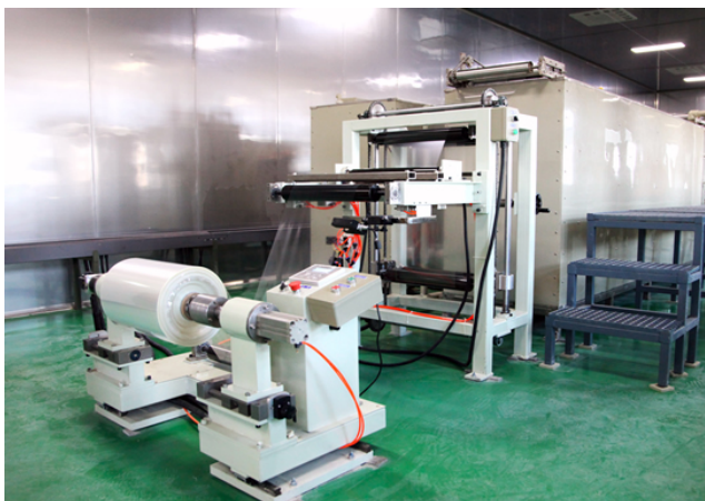
System for irradiating polymer films at the Heavy Ion Research Facility of HIRFL (Lanzhou, China)
