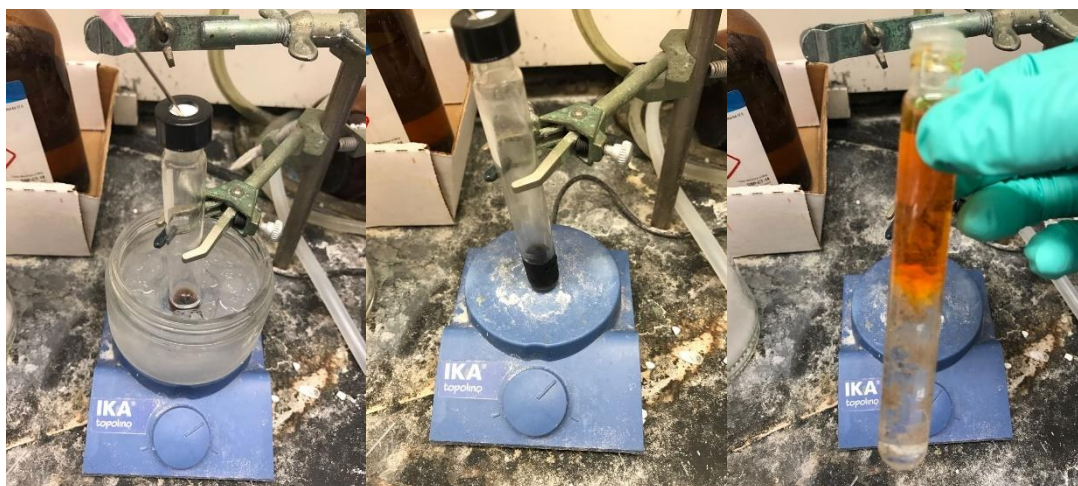
Figure S28. (Left) After addition of [B_2pin_2Me]Li complex, the mixture was stirred at 0\text{ }^\circ\text{C} for 1 h. (Center) The mixture was stirred at room temperature for another 1 h. (Right) The reaction mixture was quenched with 0.1 N HCl (10 mL) and extracted with Et_2O (5 mL \times 2).
