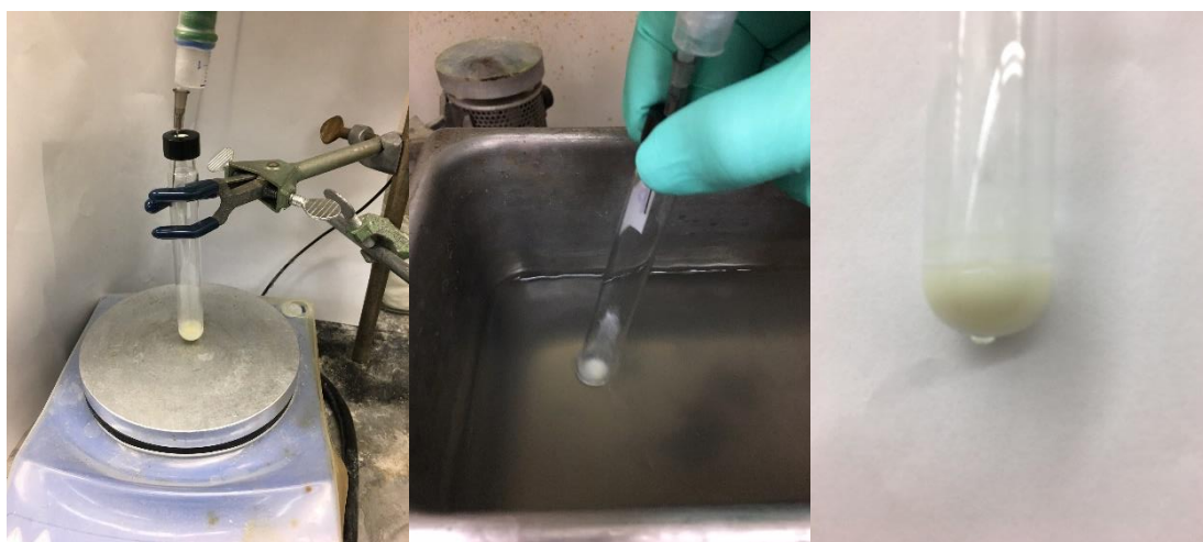
Figure S7. (Left) The mixture was stirred at room temperature until no granular \text{MgBr}_2 \cdot \text{OEt}_2 was observed ( ca. 10 min). (Center) Sonication could accelerate this process ( this was optional ). (Right) No solid was observed at the bottom of the tube.
