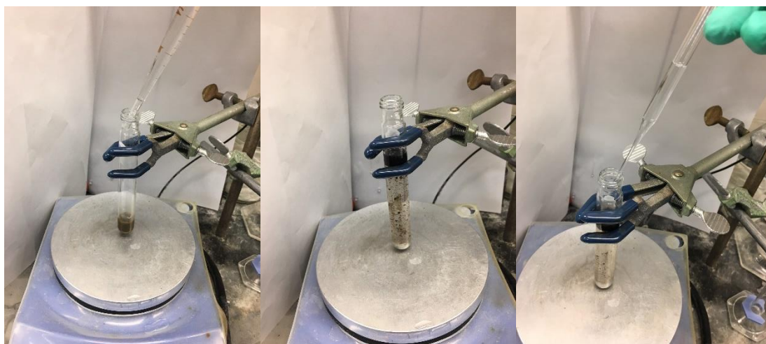
Figure S11. (Left) The reaction was quenched with 0.1 N HCl. (Center) After the addition of HCl. (Right) \text{Et}_2\text{O} was added.
