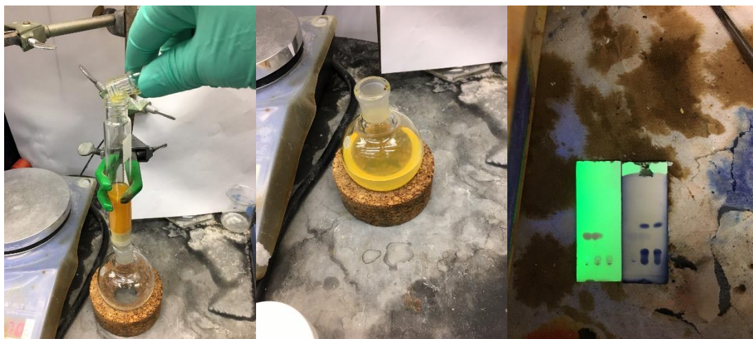
Figure S18. (Left) The diluted mixture was filtered through a short pad of silica gel and celite. (Center) The filtrate. (Right) TLC of the reaction mixture (1:20 EtOAc:hexanes). Lane 1: starting material; Lane 2: co-spot of starting material and reaction mixture; Lane 3: reaction mixture (the top spot was the desired product).
