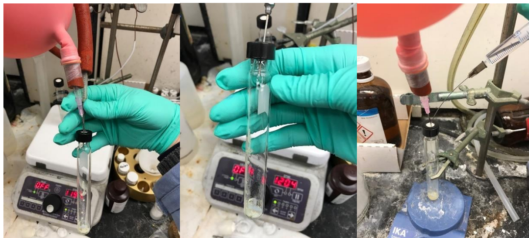
Figure S24. (Left) A screw-capped culture tube equipped with a stir bar was charged with 2-methyl-4-phenylbutanoic acid (0.2 mmol, 1.0 equiv.), tetrachloro- N -hydroxyphthalimide (0.2 mmol, 1.0 equiv.), and N,N' -dicyclohexylcarbodiimide (0.2 mmol, 1.0 equiv.). (Center) The tube was evacuated and backfilled with argon for three times. (Right) CH 2 Cl 2 was added.
