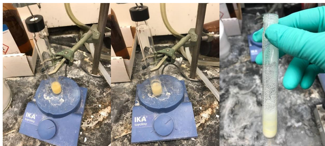
Figure S25. (Left) After addition of CH 2 Cl 2 . (Center) After stirring at room temperature for 2 h. (Right) The reaction mixture was concentrated to dryness in vacuo .
