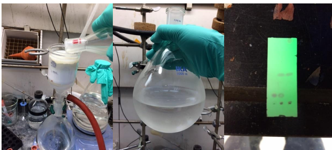
Figure S22. (Left) The diluted mixture was filtered through a pad of silica gel and celite, washed with Et_2O . (Center) After filtration. (Right) TLC of the reaction mixture (1:9 EtOAc :hexanes) under UV. (Lane 1: starting material; Lane 2: co-spot of starting material and reaction mixture; Lane 3: reaction mixture).
