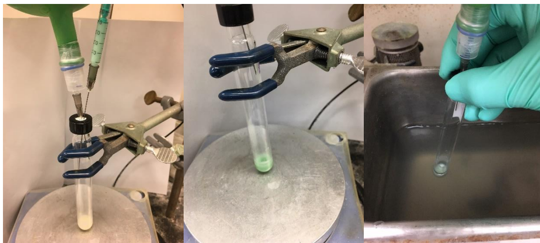
Figure S8. (Left) The suspension of \text{NiCl}_2 \cdot 6\text{H}_2\text{O}/\text{di-MeObipy} in DMF (0.05 M) was added. (Center) The mixture was stirred at room temperature until no granular \text{MgBr}_2 \cdot \text{OEt}_2 was observed ( ca. 10 min). (Right) Sonication could accelerate this process ( this is optional ).
