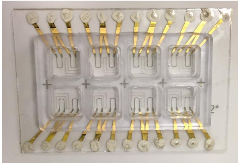
Figure S17 | 8-Well device prototype applied in initial tests and NRVM-based experiments.
