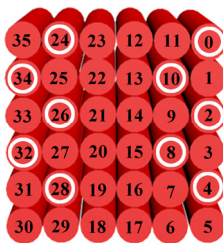
Figure S5. The locations of 10 linker strands at CU , with the base number (1 BP) and helix numbers (circle-marked sites) specified.
