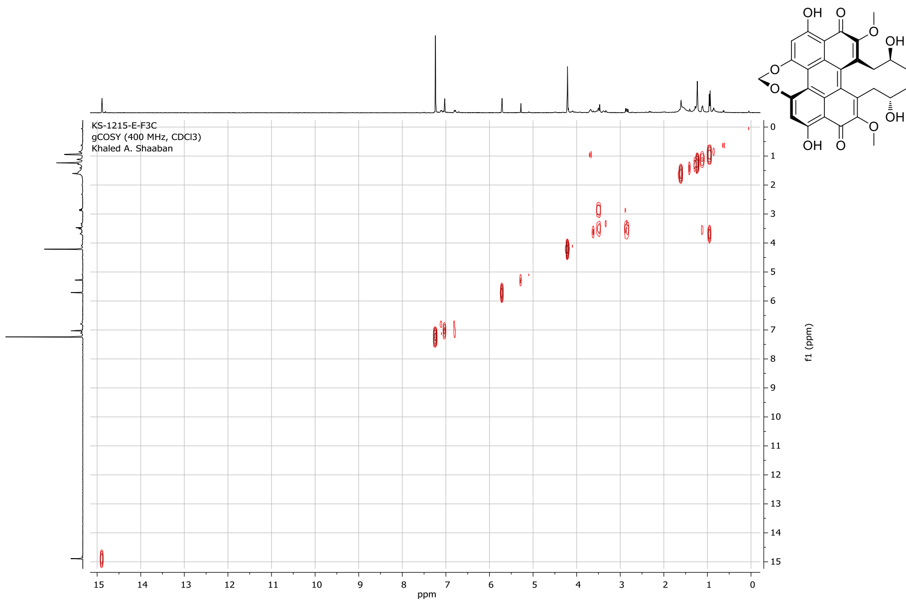
Figure. S21. ^1\text{H} - ^1\text{H} COSY spectrum ( \text{CDCl}_3 , 400 MHz) of (+)-isocercosporin ( 2 )
