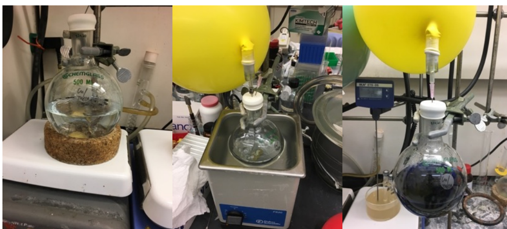
(Left) [\text{Cu}]/\text{TMEDA} solution after stirring for 5 minutes; (Center) Sparging of [\text{Cu}]/\text{TMEDA} solution with \text{O}_2 ; (Right) [\text{Cu}]/\text{TMEDA} solution after sparging for 20 minutes.
