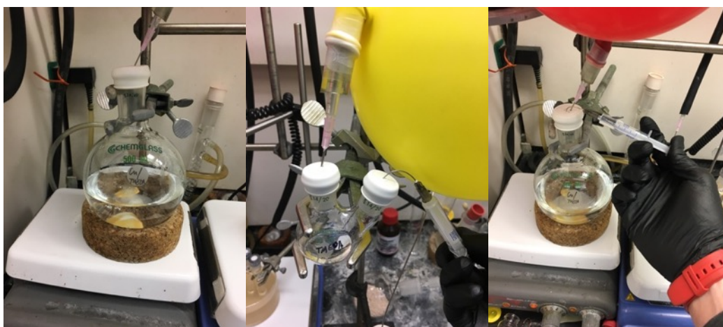
(Left) [\text{Cu}(\text{MeCN})_4][\text{PF}_6] dissolved in MeCN; (Center) Measuring out freshly distilled TMEDA; (Right) Addition of TMEDA to [\text{Cu}(\text{MeCN})_4][\text{PF}_6] solution.
