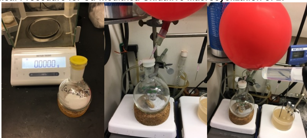
(Left) Recrystallized [\text{Cu}(\text{MeCN})_4][\text{PF}_6] ; (Center) Flask containing [\text{Cu}(\text{MeCN})_4][\text{PF}_6] for reaction; (Right) Addition of MeCN to [\text{Cu}(\text{MeCN})_4][\text{PF}_6] .
