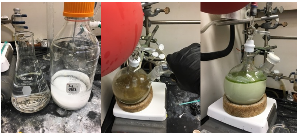
(Left) Saturated EDTA solution; (Center) Addition of EDTA solution to reaction flask; (Right) Reaction flask after addition of EDTA solution and stirring for 1 hour.
