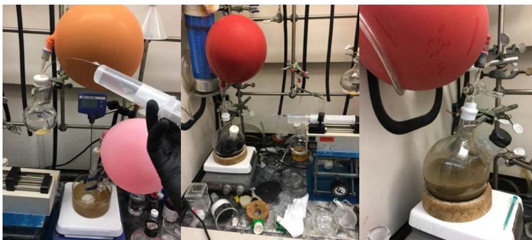
(Left) Measuring out MeCN solution of compound 2; (Center) Addition of compound 2 to reaction flask via syringe pump; (Right) Reaction flask after complete addition of compound 2.
