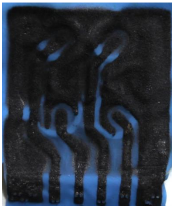
Figure S 11: Bottom of the tactile sensor. The four lines bring the signal to electronics.
