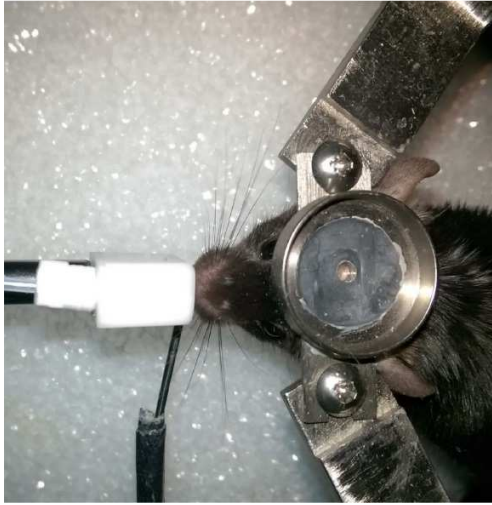
Supplementary Fig. 1: Photograph of a mouse in the olfactory VR apparatus. The mouse was head-fixed above a spherical treadmill. The head bar was ~1 inch above the treadmill, leaving enough space for the mouse to move its limbs freely. The water reward spout was positioned under the mouth. The nose chamber (white) covered the nose and snout. The nose chamber did not touch the majority of the whiskers and produced no obvious effect on whisking/grooming behavior.
