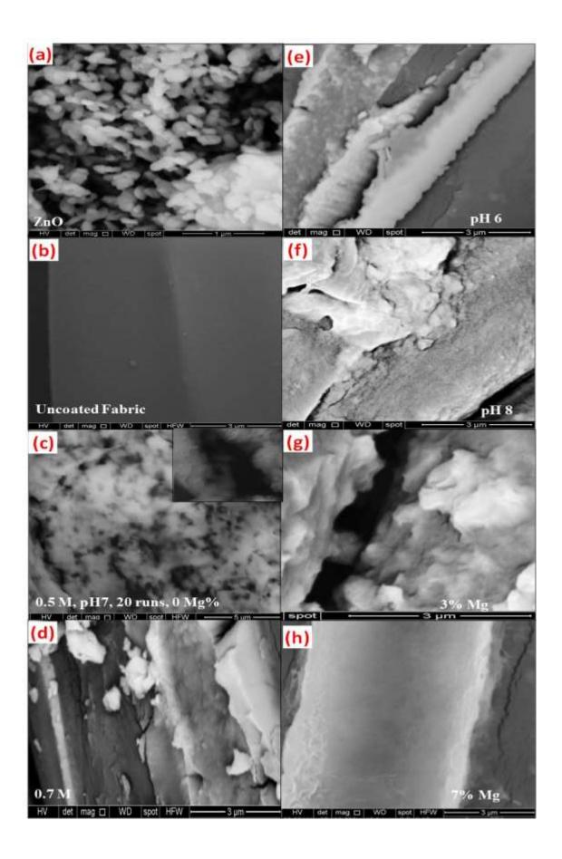
Figure S1. SEM images of (a) ZnO nanoparticles;(b) untreated cotton fabric; ZnO coated fabric at different concentrations of ZnO precursor solution: (c) 0.5 M and (d) 0.7 M at pH 7 and 20 runs; at different pH values: (e) pH 6 and (f) pH 8 at 0.5M precursor concentration and 20 runs; at different Mg doping percent: (g) 3% Mg and (h) 7% Mg at 0.5M precursor concentration, pH 7 and 20 runs.
