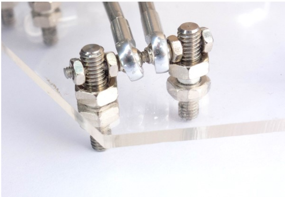
Figure S9. Rod end bearing enables smooth rotation.
