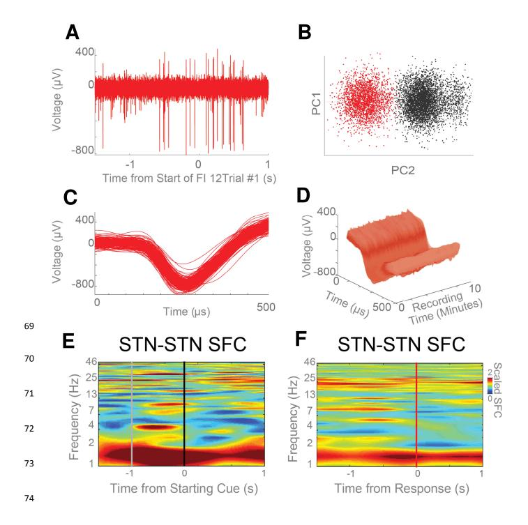
Supplementary Fig. 5. STN intraoperative human neuronal recordings. Related to Fig. 4. A) Raw voltage record at 24 kHz filtered for spikes from a single STN channel in a single patient around a single FI12 trial. B) STN neurons had consistent waveforms and were well-separated in PCA space. C-D) Waveforms were stable over the entire 10-minute intraoperative recording session. E) Spike-field coherence with STN LFPs for cue-modulated and (F) response-modulated STN neurons.
