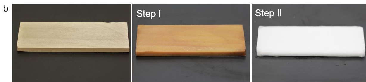
fig. S2. The lignin content and appearance between chemical processes. (a) The lignin content change (weight fraction) and overall weight loss of the initial wood specimen during chemical processing. (b) Photographic evidence showing the pure white color of the nanowood due to the high reflectivity of visible light, after the two-step chemical process.
