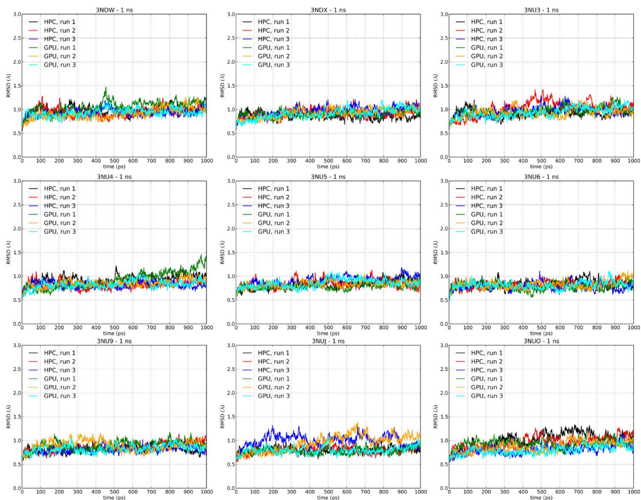
Figure S6. Comparison of RMSD values of the 1 st ns of MD simulations of the HIV1-protease system obtained by using GPU or CPU hardware.
