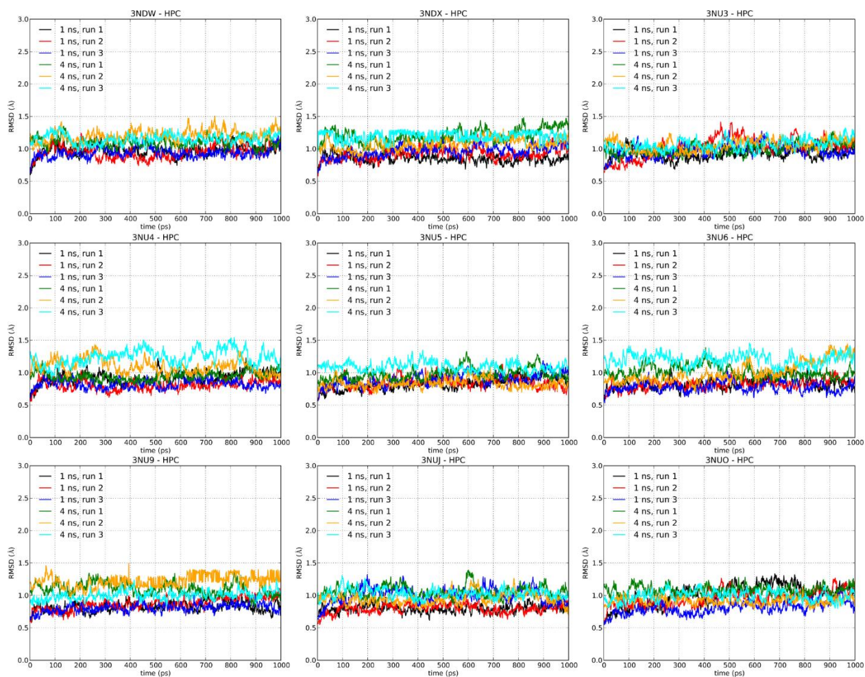
Figure S8. Comparison of RMSD values of the 1 st ns and 4 th of HPC MD simulations of the HIV1-protease system.
