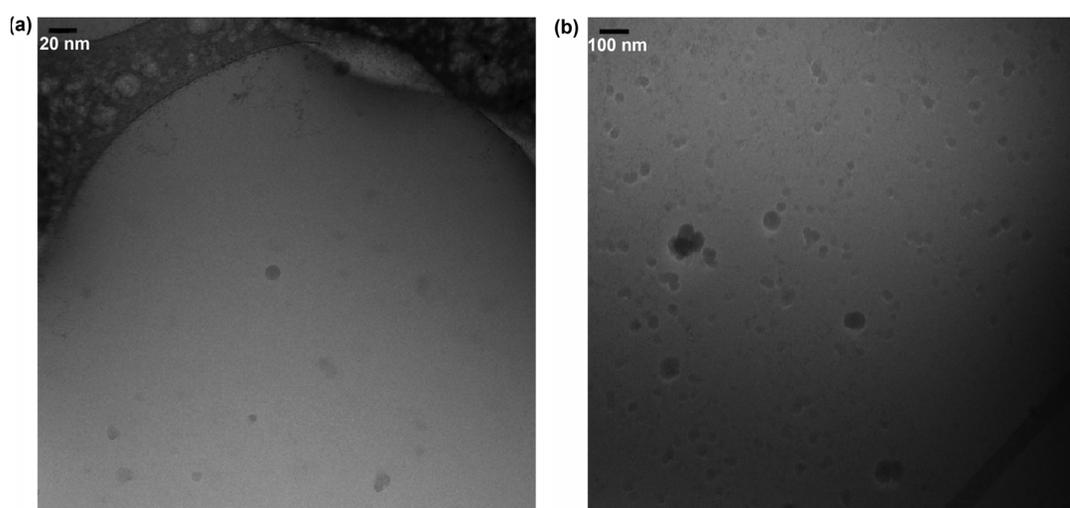
**Figure S1** Cryo-TEM images of bare and dopamine-azide coated TiO<sub>2</sub> nanoparticles. Bare TiO<sub>2</sub> nanoparticles and azide-coated nanoparticles were diluted 1:50 in distilled H<sub>2</sub>O, plunge frozen in liquid ethane and imaged. Compared to uncoated nanoparticles (a), azide-coated (b) nanoparticles and aggregate sizes appear slightly increased.
