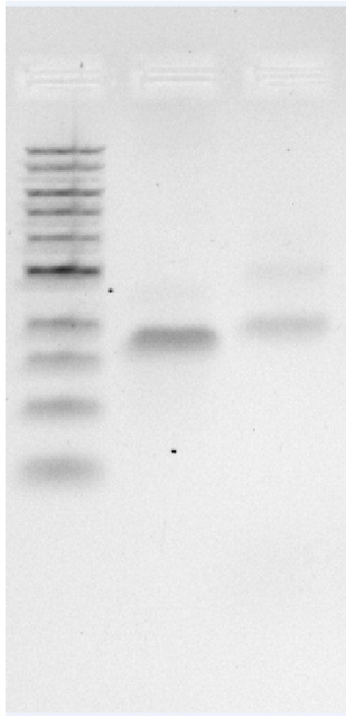
Figure S1. Agarose gel electrophoresis (1%) of DNA origami plates performed in 11 mM MgCl_2 buffered with 0.5x TBE. Lane 1: 1 kb ladder, Lane 2: p8064 scaffold, Lane 3: DNA plate with leash and pore (p8064) (from left to right).
