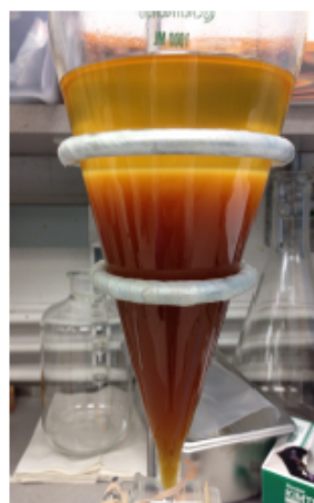
Liquid-liquid Extraction (ethyl acetate-water)
