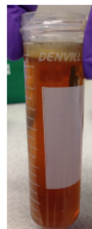
Liquid-liquid Extraction (ethyl acetate-water)
