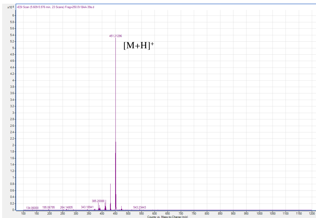
Figure S10: HR ESI negative mode spectrum of compound BAA-39a . HRMS-ESI ( m/z ): [M+H]^+ calculated for C_{24}H_{26}BF_2N_4O_2^+ : 451.21114; found: 451.21296 (4.0 ppm).
