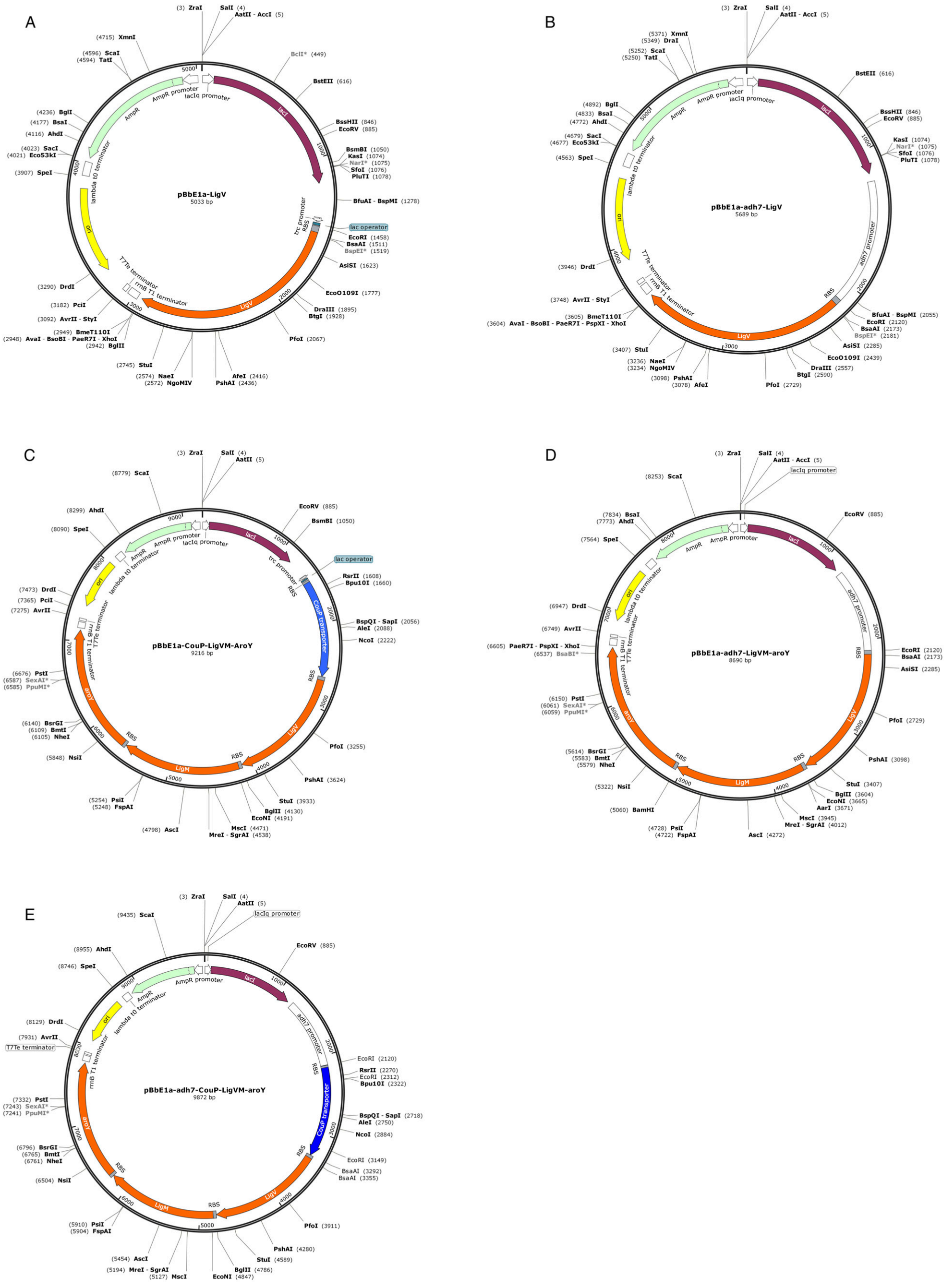
Fig. S1. Plasmid maps of the constructs in this study: (A) pBbE1a-LigV, (B) pBbE1a-adh7-LigV, (C) pBbE1a-CouP-LigVM-aroY, (D) pBbE1a-adh7-LigVM-aroY, and (E) pBbE1a-adh7-CouP-LigVM-aroY.
