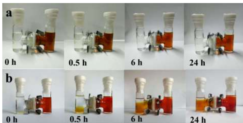
Figure S9. Digital photos of H-type cells separated by NCP-CPE a) and PP separator b).
