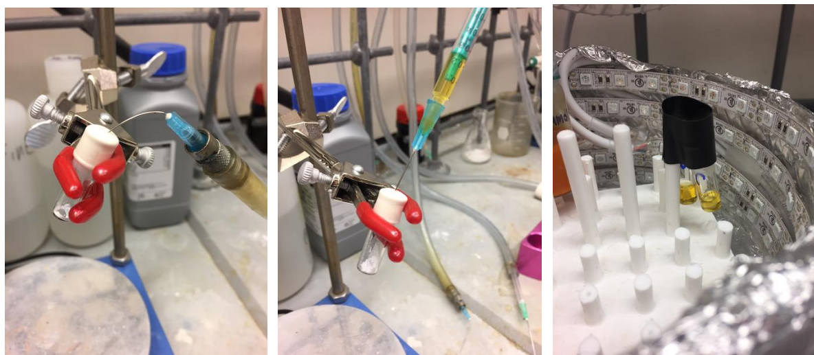
Figure SI- 3. (a) Vial containing 0.68 μmol of peptide in a sealed and Parafilm-wrapped vial with Schlenk line undergoing vacuum/Ar cycles. (b) Schlenk line has been removed, and the DMF stock solution is contained within the syringe just before injection. (c) Two reactions side-by-side (conveniently fastened by electrical tape...not essential) in the photoreactor (turned off, fan present) in close proximity to the LED source.
