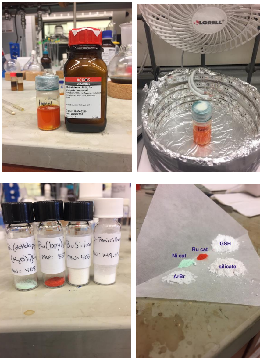
Figure SI- 2. (a and b) 1.0 mmol (307 mg) scale reaction shown for the Ni/photoredox thioarylation reaction employing glutathione. Similar reaction vial and setup were applied to the gram scale reaction, using the same blue LED photoreactor. (c and d) All the necessary reagents weighed out on the benchtop in the air, before direct addition to the reaction vial.
