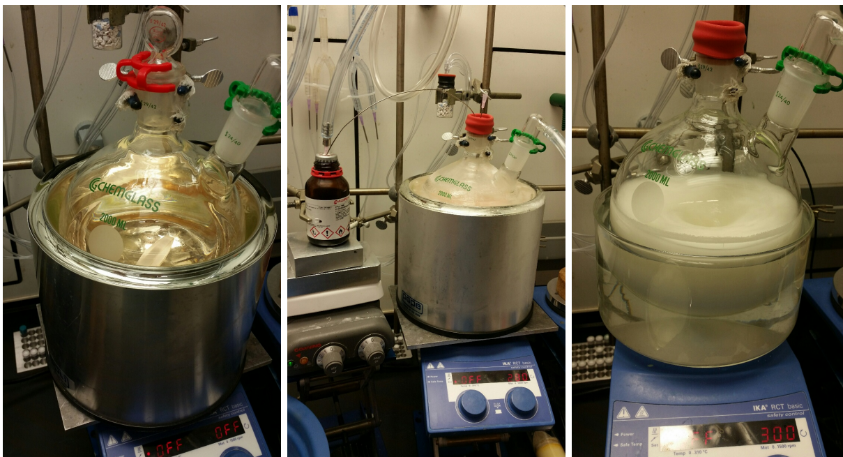
(Left) Dimethylamine in THF added to 500 mL of diethyl ether. (Center) Reaction flask cooled to -78\text{ }^{\circ}\text{C} and n -butyllithium solution added via cannula. (Right) Warming the reaction to room temperature forms a white slurry.
