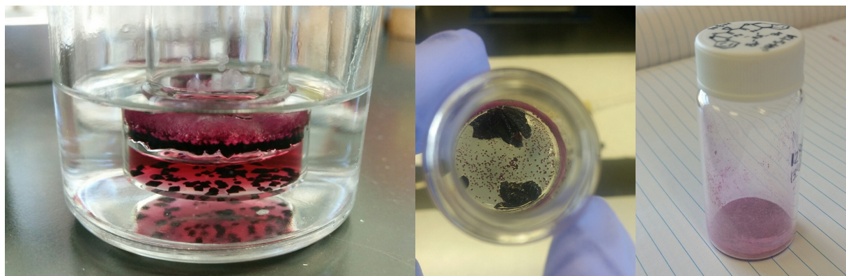
(Left) Crystallized 4b following vapor diffusion. (Center) Large crystals of 4b . (Right) The powdered form of 4b after crushing the crystals with a spatula and drying under vacuum.
