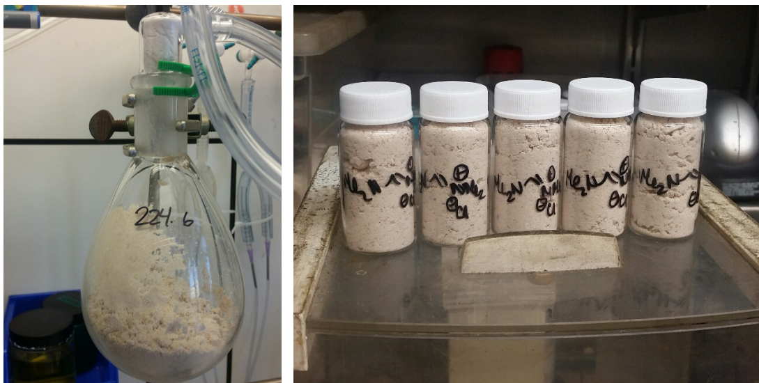
(Left) Drying the salt under vacuum. (Right) Dried formamidinium salt stored in the glovebox.
