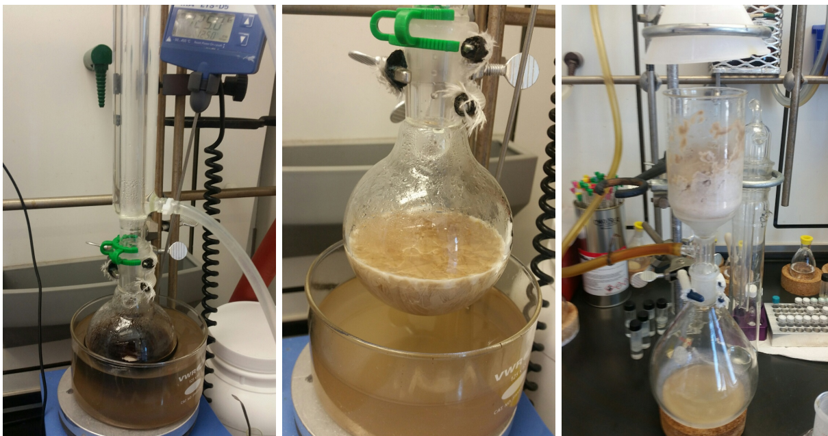
(Left) Reaction after heating for 3 days. (Center) Precipitated salt after cooling the reaction flask. (Right) Filtering the salt under a flow of argon.
