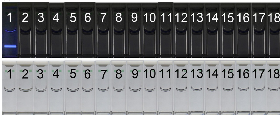
Fig. S11. Digital images of DBB-NO (5 \mu M) upon addition of various competitive species after 15 min under 750 nm femtosecond laser irradiation. (1) DEA·NONOate, (2) DBB-NO only, (3) AA, (4) MGO, (5) DHA, (6) \text{NO}_2^- , (7) \text{ONOO}^- , (8) \text{NO}_3^- , (9) \text{H}_2\text{O}_2 , (10) \text{HClO} , (11) \cdot\text{OH} , (12) ^1\text{O}_2 , (13) cysteine (Cys), (14) glutathione (GSH), (15) \text{Fe}^{3+} , (16) \text{Ca}^{2+} , (17) \text{K}^+ , (18) \text{Na}^+ .
