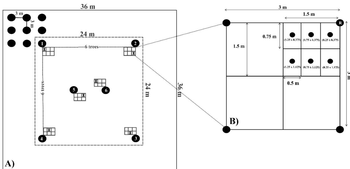
**Supplementary Figure S1.** Soil and litter sampling based on Voronoi grids. A) total plot area (36 x 36 m), the useful plot (24 x 24 m) and spacing between plants (3 x 3 m). Numbers 1 to 6 indicate the trees selected for sampling and "X" indicates the collection points at each tree; B) "R" represents the reference tree and the six rectangles represent the dimensions of each sampling point.
