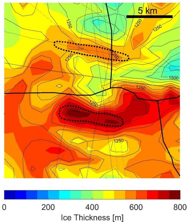
**fig. S2. Interpolated ice thickness near the DIC summit area.** The ice thickness is overlain on bedrock elevation contours [m asl.]. Fine black lines indicate the location of the radar transects, whereas the thick black lines represent the ice divides. The locations of the subglacial lakes are indicated with dotted lines.
