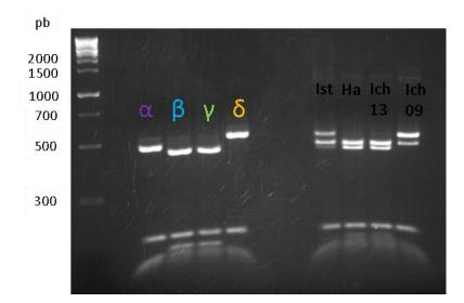
**Supplementary Figure 3.** Unprocessed gel image of double digestion with Taqa1 and Ban1 of a 1267–1276 bp fragment of *cidB* gene which was amplified with primers 7/8 related to Figure 8c.
