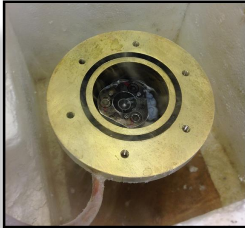
Supplementary Figure 2: Cryogenic loading chamber set up: a) side view showing the brass coils through which the gas is pumped into the chamber, b) top view showing the inside of the chamber with a DAC immersed in liquid \text{CH}_4 , with the whole set up surrounded in liquid nitrogen in a polystyrene box.
