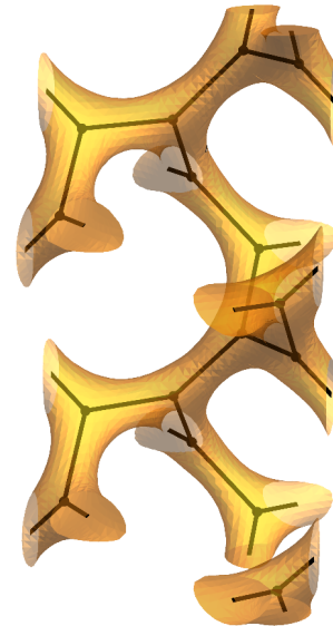
Fig. 1. Skeletal graph of a single gyroid. We show two repetitions of a (non-primitive) cubic cell of a single gyroid, along with the associated skeletal graph (in black).
