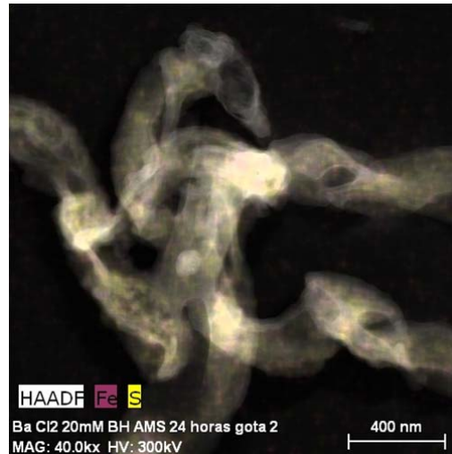
Fig. R1. HAADF images obtained by HRTEM showing bacteria from the biofilms ( I. loihiensis MAH1) and EDX maps showing the S and Fe distribution.
