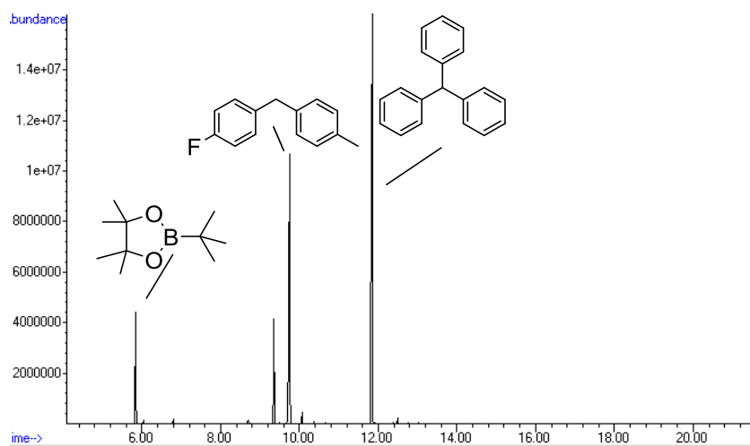
Figure S 32: GCMS chromatogram of the crude from the reaction to produce 3m
