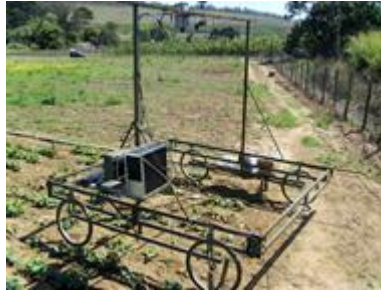
Figure 5: Photo of the Canopy Reflectance Spectra acquisition process using a platform with wheels.
