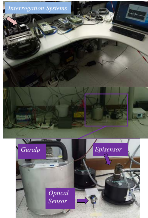
Figure S7 Experimental configuration for optical sensor characterization from the ground through the shaking table method
