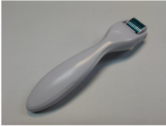
Figure S1. The picture of the commercial microneedle roller (DRS Dermaroller System 600, Derma Roller System, Ltd., Germany). There are 10 rows on the head, with 60 needles per row. The space between rows is 2 mm. The derma roller comes in several different needle lengths depending on the treatment. In this paper, 0.5-mm-long, 1.0-mm-long and 1.5-mm-long models are used.
