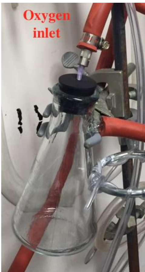
Figure SI-4. Anti-suck-back trap.
