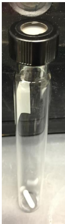
Figure SI-1. Reaction apparatus for dearomatization reactions: glass culture tube with threaded end (20 x 125 mm; Fisher scientific part # 14-959-35A), phenolic screw-thread open-top cap (Kimble-Chase part # 73804-15425), PTFE-lined silicone septum (Thermo Fisher scientific part # B7995-15), and a small PTFE-coated stir bar. Note that some dearomatization procedures call for a slightly longer culture tube (20 x 150 mm; Fisher scientific part # 14-959-37C).
