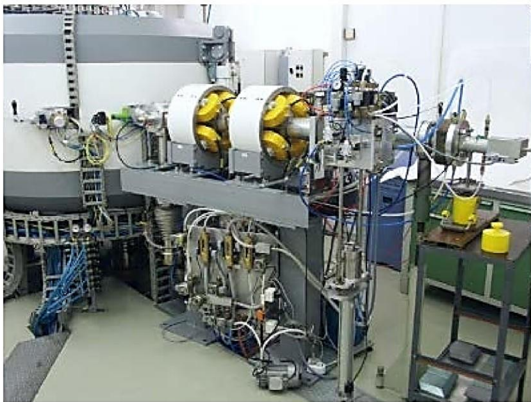
Figure S2. View inside the cyclotron of the HZDR Research Site Leipzig (Cyclone 18/9, IBA Radiopharma Solutions, Belgium). More information on the cyclotron can be found at: http://www.iba-radiopharmasolutions.com .
