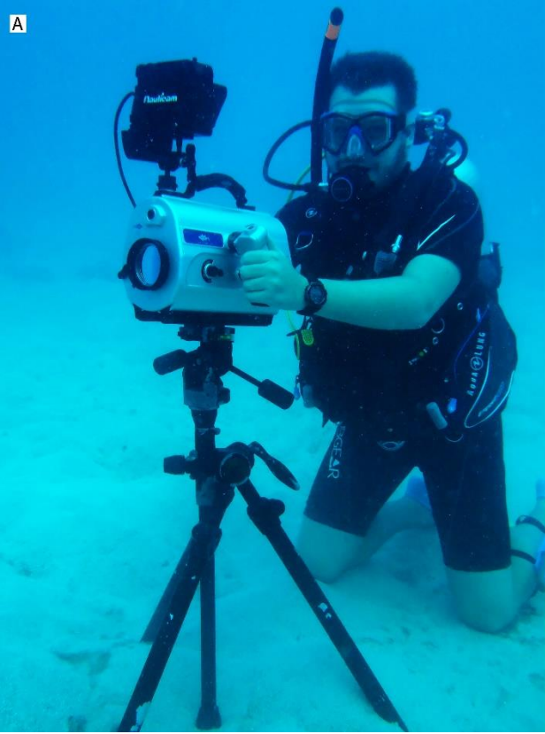
fig. S3. Camera hardware in use. (A) Underwater polarization camera prepared for recording sun inference data. (B) Underwater polarization camera with fish-eye lens, in a configuration similar to how the sensitivity data were collected.
