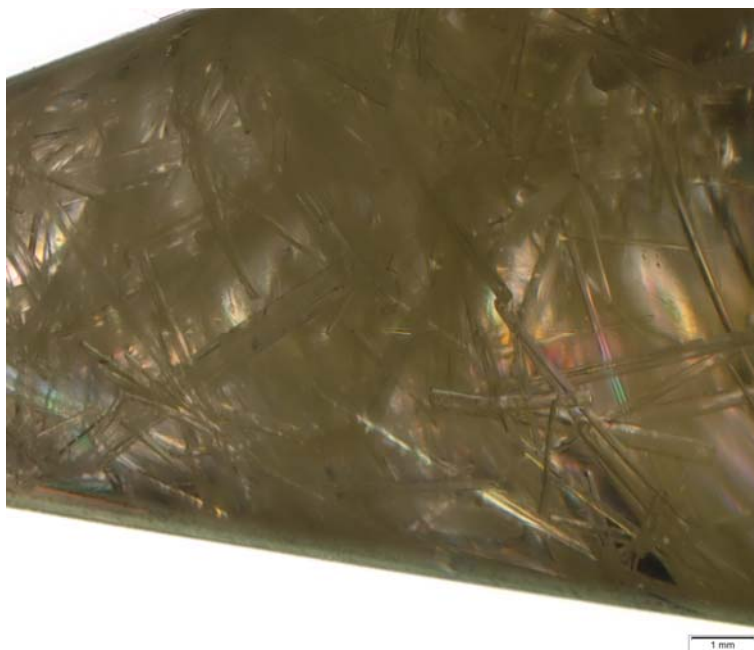
Supplementary Figure 20: Microscope picture of crystals grown in a 15 ml polypropylene centrifuge tube by mixing 1 ml of a 0.62 M solution of (1 S ,2 R )-(+)-ephedrine hydrochloride and 1 ml of a 5.34 M solution of sodium iodide. The scale bar corresponds to 1 mm.
