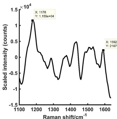
**Figure S5.** The tracking of dye 823 nanotag solution through 25 mm of tissue following a scaled subtraction. The peaks at 1178  $\text{cm}^{-1}$  and 1592  $\text{cm}^{-1}$  are revealed. This approach removes signal collected at the zero position (tissue) from that collected at the 8 mm offset (tissue and dye). All measurements were carried out using a 2 s integration time, 5 accumulations, 830 nm laser excitation wavelength.
