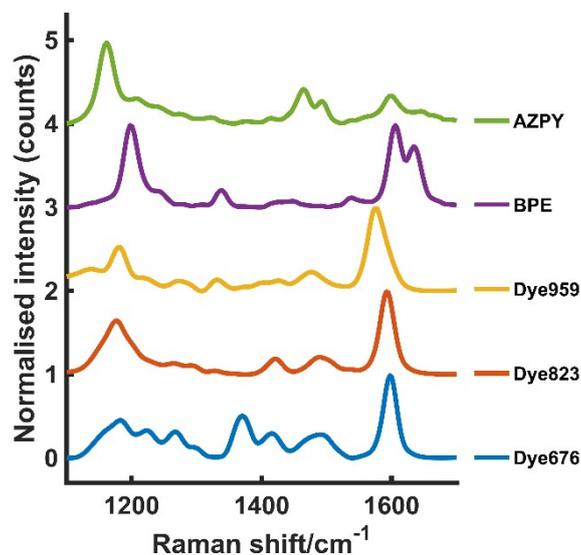
**Figure S2. SERS spectra of the five Raman reporters used in this work. Dyes 676, 823 and 959 are chalcogen based reporters BPE and AZPY are commercially available. Spectra were obtained using the SORS instrument in a conventional Raman mode. Dyes 1 – 3 are resonant at 676, 823 and 959 nm respectively. BPE and AZPY are non-resonant molecules. All measurements were carried out using a 2 s integration time, 5 accumulations, 830 nm laser excitation wavelength.**
