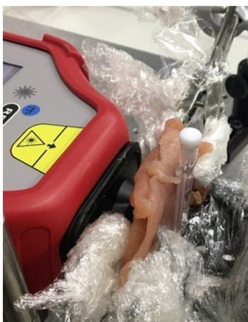
**Figure S3. Experimental set-up using a handheld SORS spectrometer for the detection of nanotags through tissue. Nanotag solutions were held in a cuvette and the cuvette was placed behind tissue samples. The nose cone was brought into contact with the tissue ensuring there was no space between the tissue sample and the instrument.**
