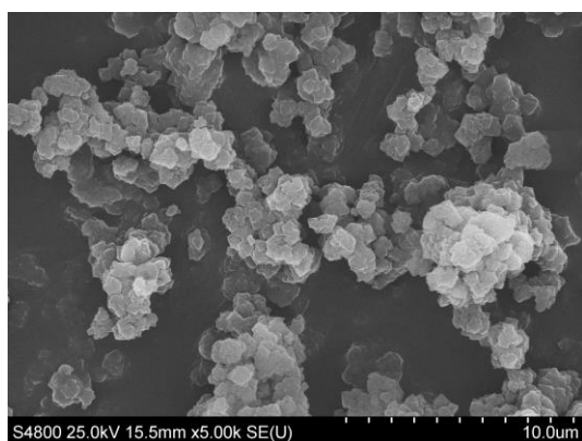
Figure S11. SEM images of as synthesized 1-SO 3 H (top), 1-SO 3 Na (bottom). Particles retain their morphology and size distribution (0.2 – 1 μm).
