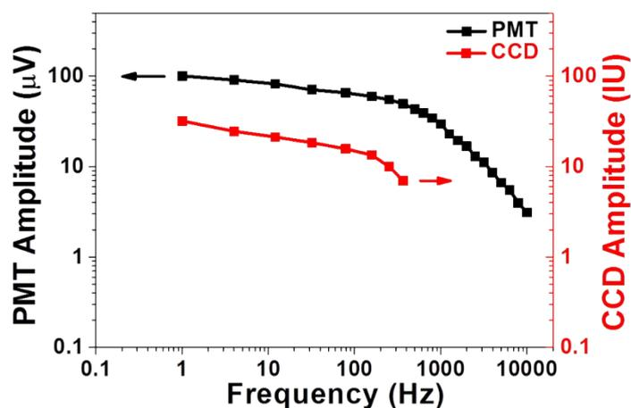
**Figure S5.** EIS spectrum of a single AuNR recorded by CCD (red curve) and PMT (black curve), respectively. Note the unit of CCD amplitude is Intensity Unit (IU) from gray-scaled camera image. That of PMT amplitude is the voltage (mV or  $\mu\text{V}$ ) across a transistor when photocurrent passes through it.
