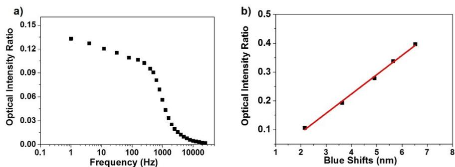
**Figure S11.** a) Changes of optical intensity ratio of a single AuNR under electrochemical charging and discharging. b) The linear relationship between the optical intensity ratio and the wavelength blue shifts.
