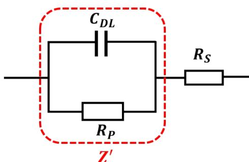
**Figure S8.** Randles equivalent circuit of the electrochemical cell.
