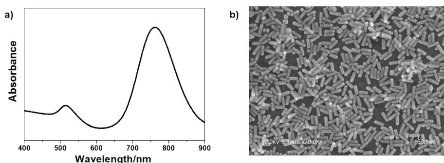
**Figure S1.** a) and b) UV-Vis absorbance spectrum and SEM image of the synthesized AuNRs, respectively.
