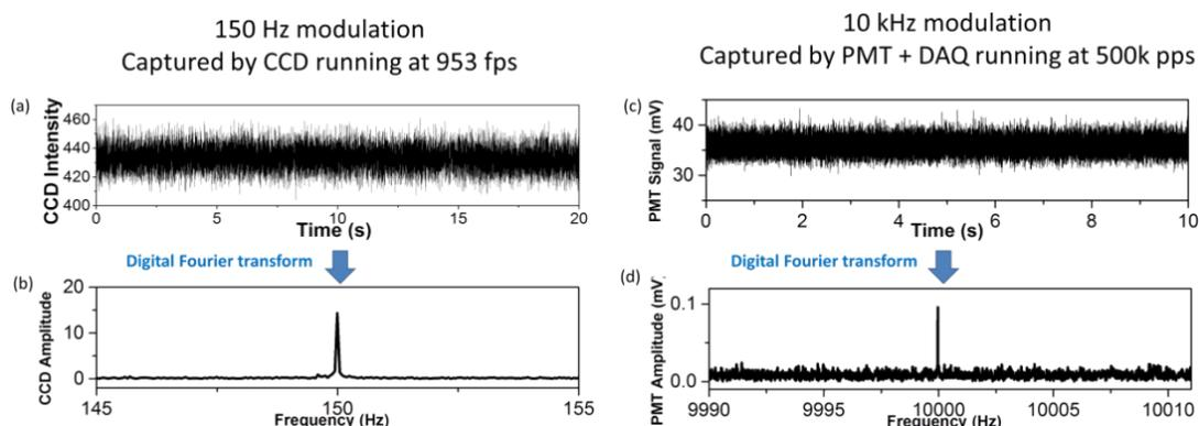
**Figure S3.** Original intensity curves (a, c) and the corresponding Fourier transform of a single AuNR under the potential modulation of 150 Hz (a, b, captured by CCD) and 10 kHz (c, d, captured by PMT and digital acquisition device, DAQ), respectively. Note the unit of CCD amplitude is Intensity Unit (IU) from gray-scaled camera image. That of PMT amplitude is the voltage (mV or  $\mu$ V) across a transistor when photocurrent passes through it.
