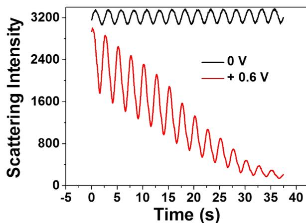
**Figure S4.** Both the scattering intensity and its fluctuation amplitude decreased when applying a positive potential to induce the oxidation of a single AuNR. A 0.4 Hz sine wave modulation with the peak-peak voltage of 1 V is applied. The offset is  $-0.5$  V (sweeping between  $-1$  V and 0 V) in black curve. It is  $+0.1$  V (sweeping between  $-0.4$  V and  $+0.6$  V) in the red curve.
