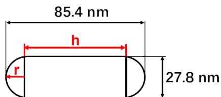
**Figure S10.** The length and width of the synthesized AuNRs.
