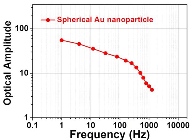
**Figure S9.** Representative EIS spectrum of a single spherical Au nanoparticle (diameter 70 nm).
