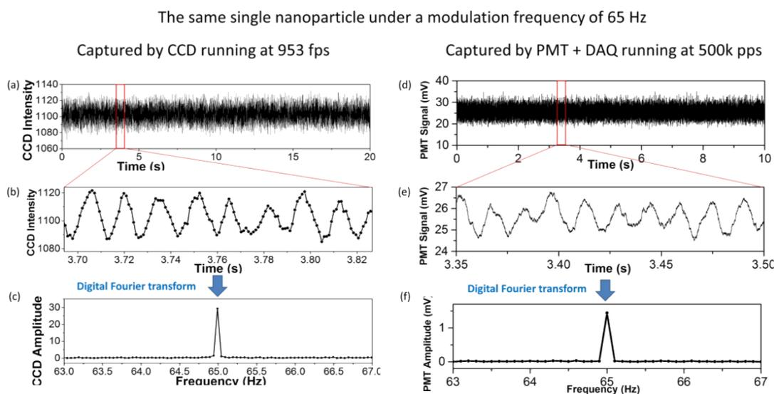
**Figure S6.** Original (a, d) intensity curves, zoom-in curves (b, e) and the corresponding Fourier transform results (c, f) of the same single AuNR under a modulation frequency of 65 Hz. Note the unit of CCD amplitude is Intensity Unit (IU) from gray-scaled camera image. That of PMT amplitude is the voltage (mV or  $\mu\text{V}$ ) across a transistor when photocurrent passes through it.
