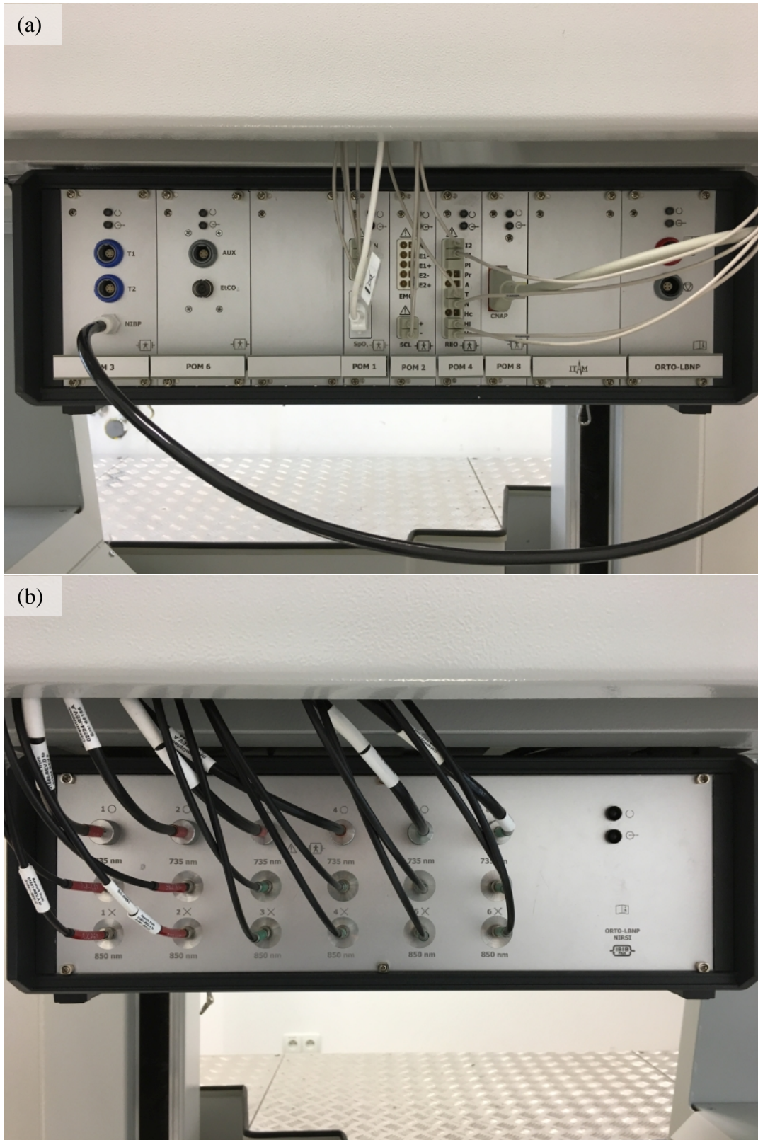
Figure S15. Medical monitoring subsystem: the (a) main module box by the Institute of Medical Technology and Equipment , Poland, (b) in-house-designed NIRS module box by the Nalęcz Institute of Biocybernetics and Biomedical Engineering of the Polish Academy of Sciences .
