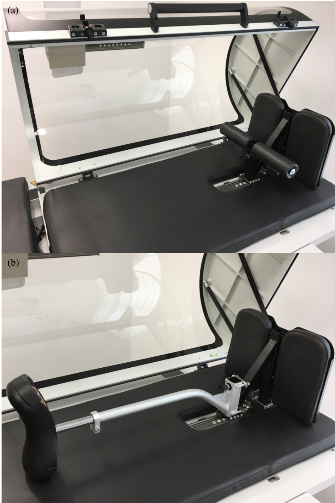
Figure S18. Photographs of the prototype system: (a) open LBNP chamber with the footboard, (b) optionally mounted saddle.
